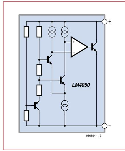
Figure 2. Block diagram of the LM4050 precision zener.
